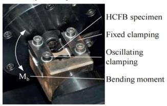
**Fig. 8** High cycle fatigue bending test setup for wire-EDM samples and broached samples [34]
