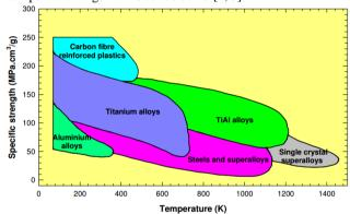
**Fig.1**Temperature dependence of specific strength of various groups of alloys [3]
