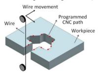
Fig. 4 Mechanism of wire-EDM
