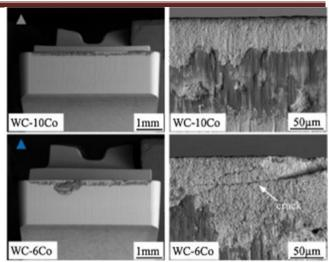
Fig. 3 Tool wears in orthogonal cutting of Inconel [19]
