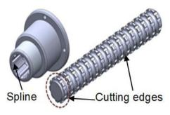
**Fig. 2** Spline cut from broach tool with multiple cutting edges Broaching has been used for cutting complicated fir tree slots in jet engines. In past, due to a lack of alternative, manufacturers had to live with the following limitations of this process that rendered it a costly operation:
