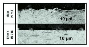
**Fig. 6**White layers in main cut eliminated in fourth trim cut, Inconel [26]
