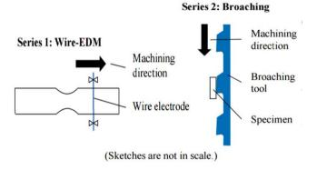
**Fig. 7** Preparation of fatigue test samples for wire EDM and broaching [34]
