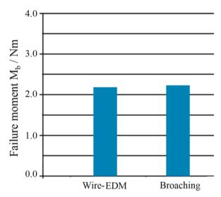
**Fig. 9** Comparable fatigue failure moment for wire-EDM samples and broached samples [34]
